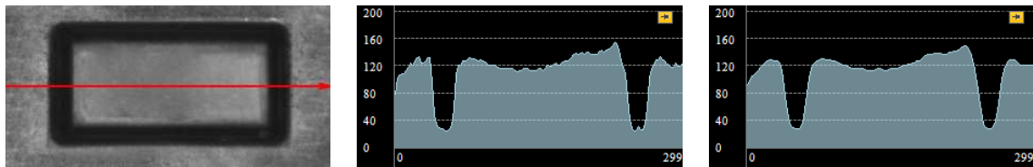
The image is scanned along the path and the brightness profile is extracted and smoothed.
